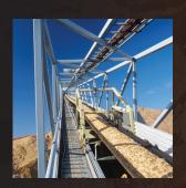
Mulhern Belting's 5-3802 features a strong 3-Ply 600 lbs PIW carcass, a smooth top cover and a bare bottom cover. The stout 3/8" thick top cover is moderately oil resistant and the bare bottom cover makes this a heavy duty slider-bed friendly belt. 3-Ply 600 3/8" x Bare is especially well-suited for the wood industry.
